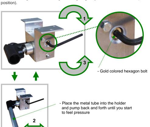
**4.** Refill the oil reservoir of the hydraulic pump-unit with oil and close. (add oil until the oil runs out of the filling hole)
