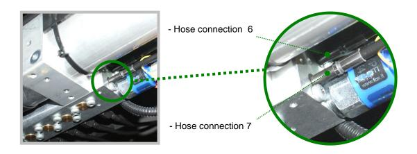
Note: Remove the protective plastic sleeves that are placed over the hydraulic nipples just before actual installation on the pump-unit, to avoid unnecessary dirt, or damage to the nipples.
