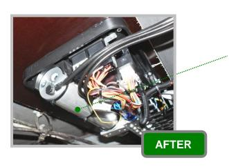
Casing of installation box removed, the hydraulic pump-unit will be accessible
